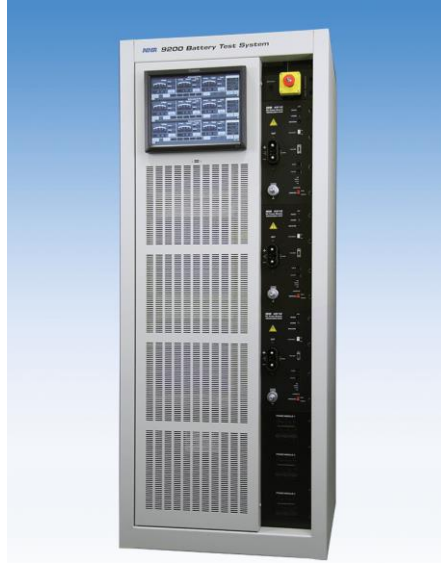
Figure 2.2b: CE-CERT monitoring device (NHR Battery Pack Test System – 9200 series)
