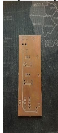
Figure 4.1.13c: Top layer of test circuit printed by EE shop in Chung Hall
