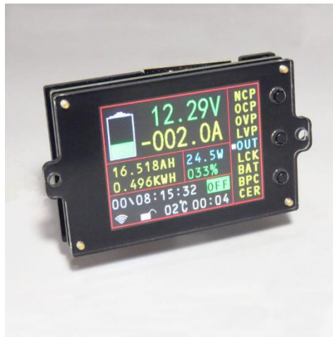
Figure 2.2c: Wireless battery monitoring systems such as these are able to be purchased and used by almost anyone, but still fails to address the aforementioned issues
