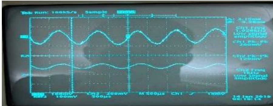
Figure 10.2.1: Oscilloscope output for the current (Top) and input voltage (Bottom).
